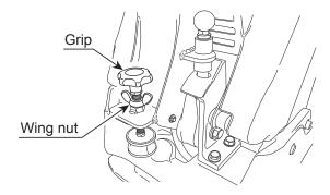
Figure 10. Handle Height Adjustment
